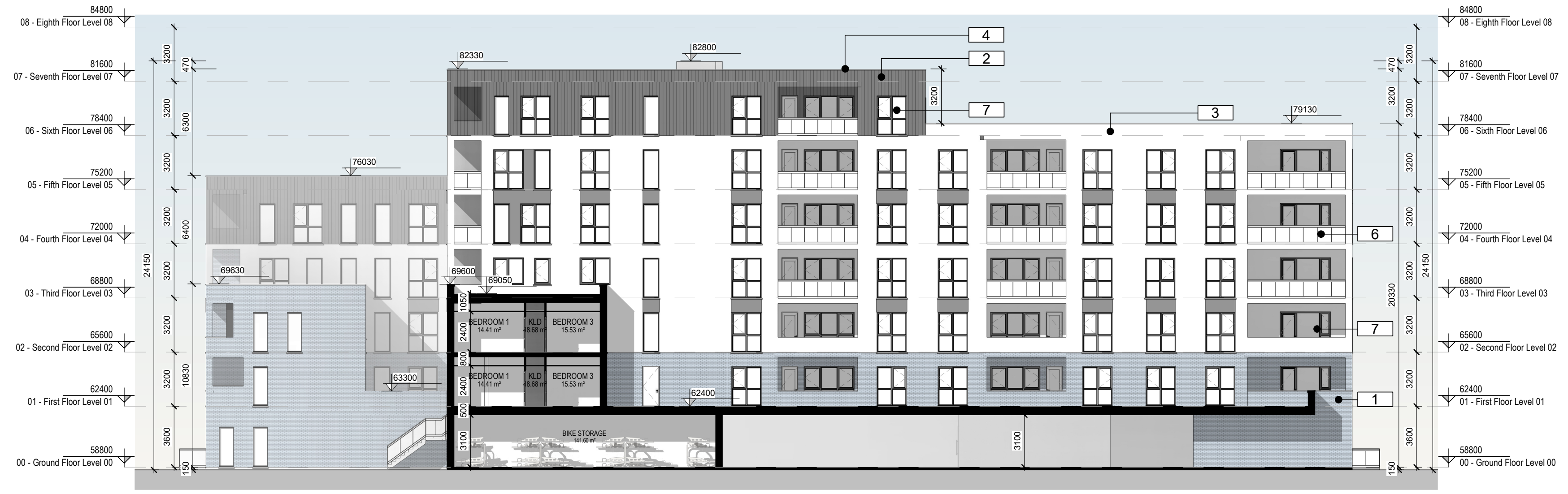
1 A4 BLOCK EAST ELEVATION
